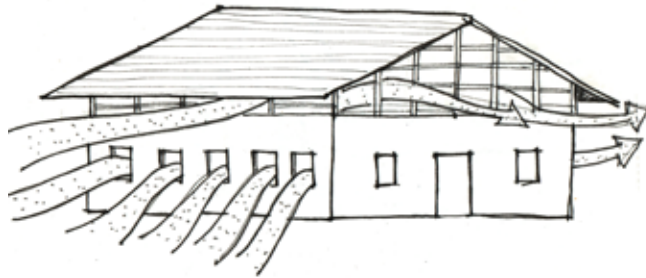
Illustration showing verandahs, openings at the roof, window and door openings for ventilation purposes
